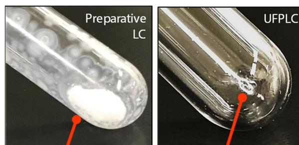
**Fig. 7 Conditions of Ibuprofen Fractions after Drying**
