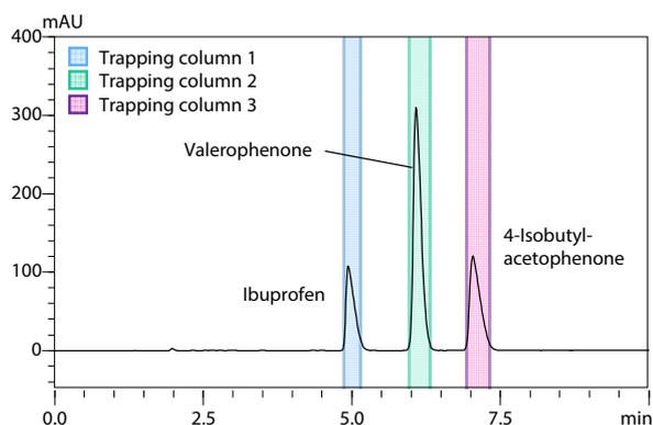
**Fig. 4 Preparative LC Chromatogram of Ibuprofen and Its Analogs (UFPLC)**
