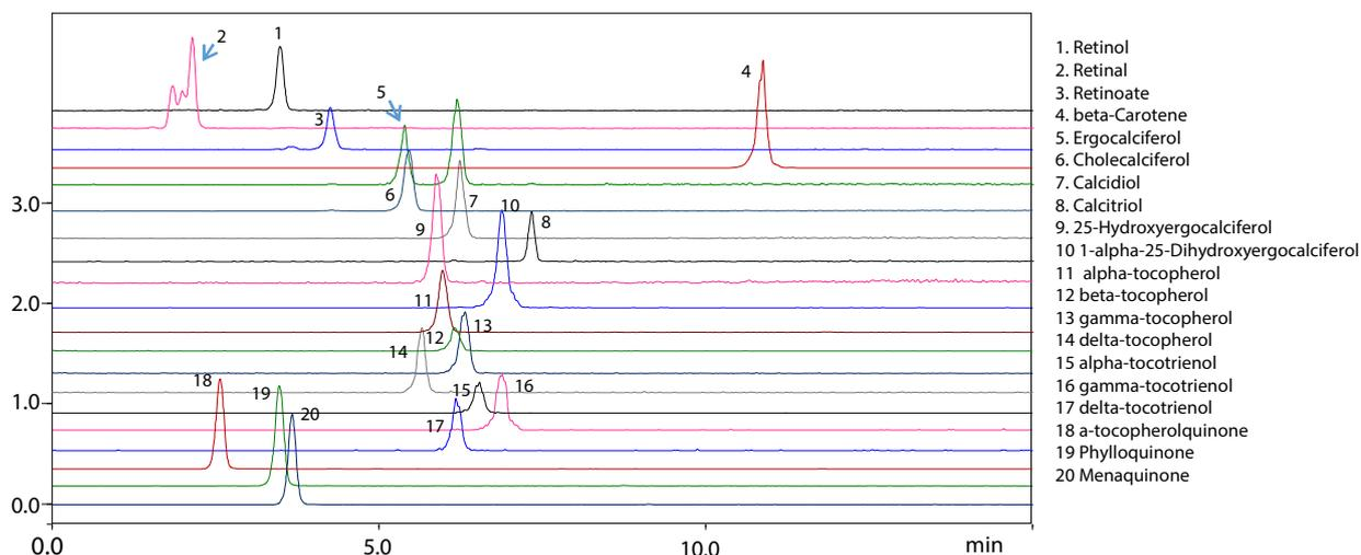
**Fig. 1 Chromatogram for Standard Solutions (1 µmol/L)**
