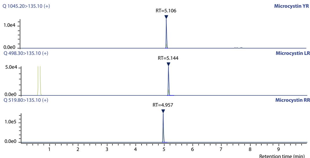
**Fig. 1 Chromatogram of 1 µg/L Standard Samples**
