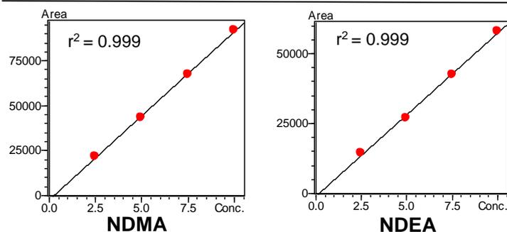
Figure 2: Calibration Curves from 2.5 ppb to 10 ppb
