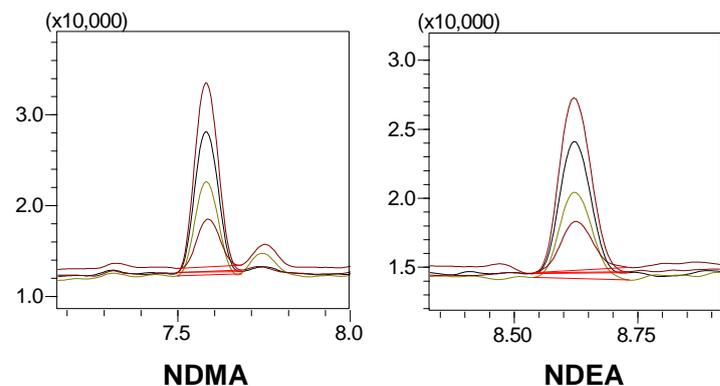
Figure 3: Chromatographic overlay from 2.5 ppb to 10 ppb
