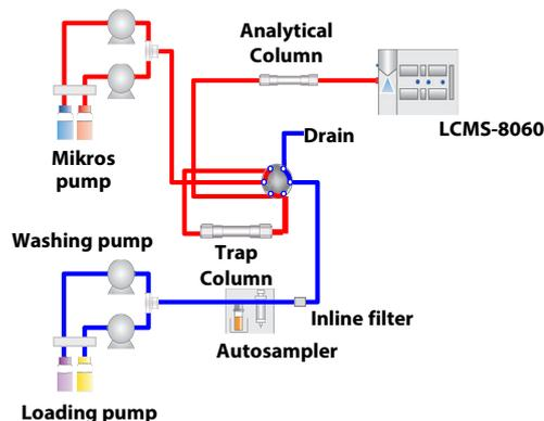
Fig. 2 Flow Diagrams of Trap and Elute System
