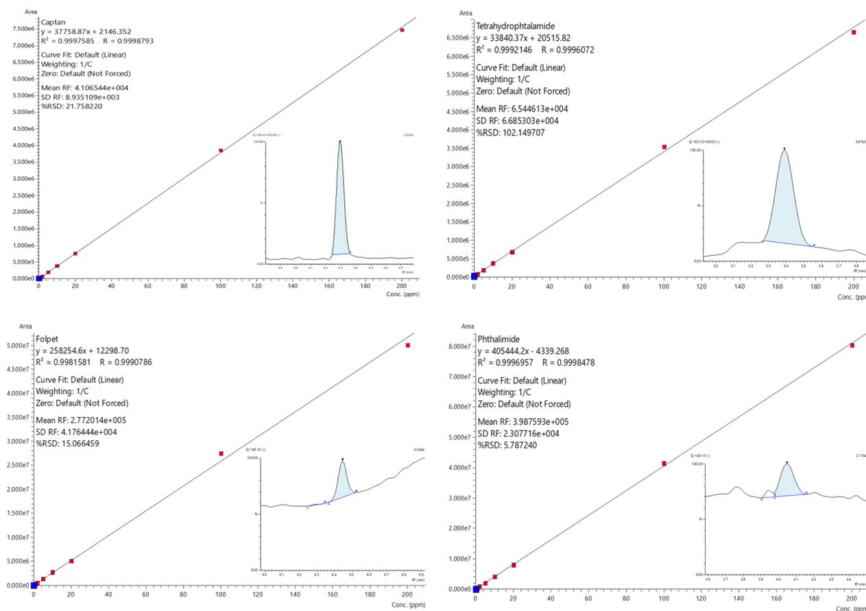
Fig. 3 Calibration Curves and Chromatograms at 0.1 ng/mL
