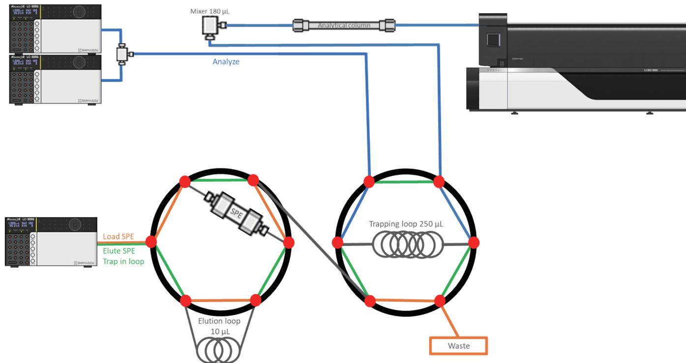
Figure 3 Setup of the on-line SPE analytical system
