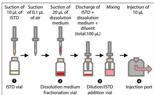
Fig. 5 Flow of Internal Standard (ISTD) Addition by Autosampler
