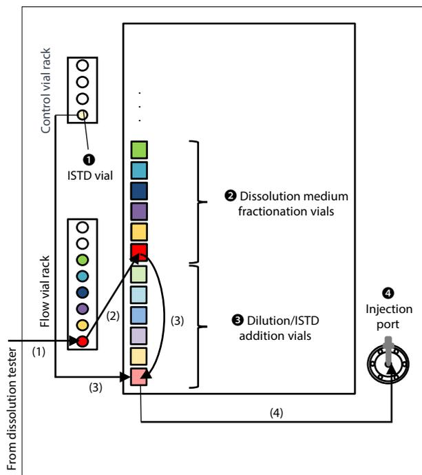
Fig. 4 Example of Vial Arrangements in Autosampler
