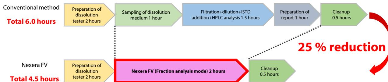
Fig. 1 Comparison of Workflow of Online Dissolution Testing\*2
