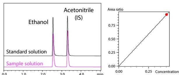
Fig. 5 Chromatogram for Alcohol Concentration Measurement (FID)
