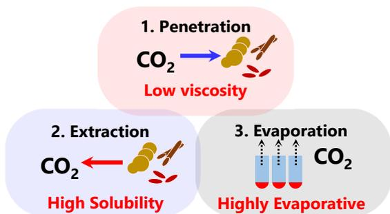
Fig. 1 Unique features of SFE (Supercritical Fluid Extraction)
