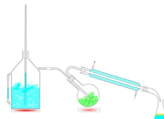
Fig. 4 Steam distillation
