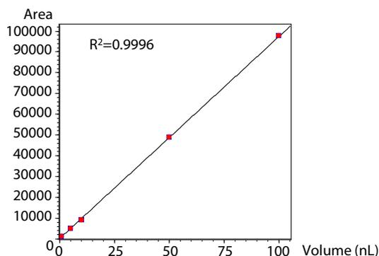
**Fig. 1 Calibration Curve of Hydrogen (1, 5, 10, 50, 100 nL)**
