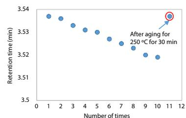
Fig. 6 Shift in Retention Time of Methane Over a Number of Measurements
