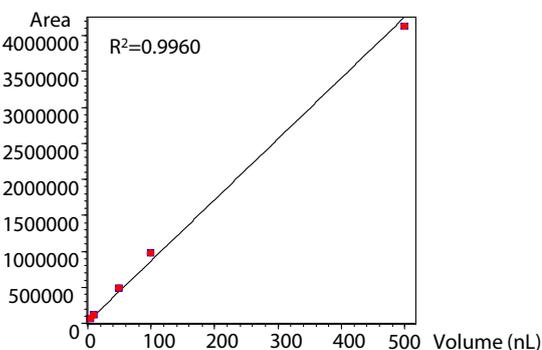
**Fig. 2 Calibration Curve of Methane (5, 10, 50, 100, 500 nL)**
