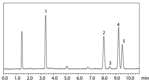
Fig. 2 Class 1 Standard Solution Chromatogram (Water-Soluble Sample) Using Procedure A
