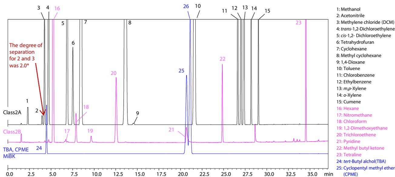
Fig. 8 Class 2 Standard Solution Chromatogram (Water-Soluble Sample) Using Procedure A with N<sub>2</sub> Carrier Gas
