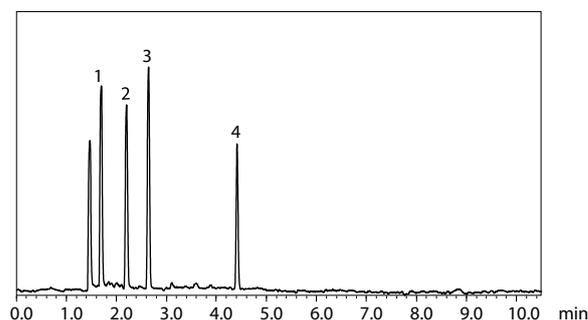
Fig. 3 Class 1 Standard Solution Chromatogram (Water-Soluble Sample) Using Procedure B
