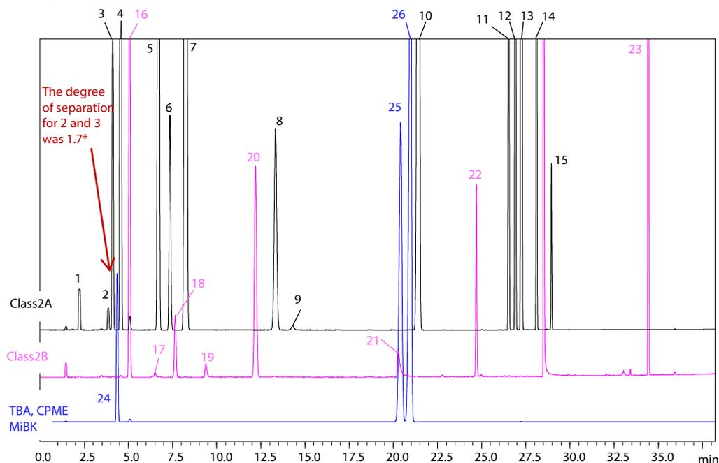
Fig. 4 Class 2 Standard Solution Chromatogram (Water-Soluble Sample) Using Procedure A
