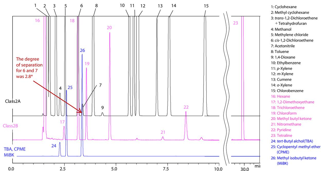
Fig. 5 Class 2 Standard Solution Chromatogram (Water-Soluble Sample) Using Procedure B
