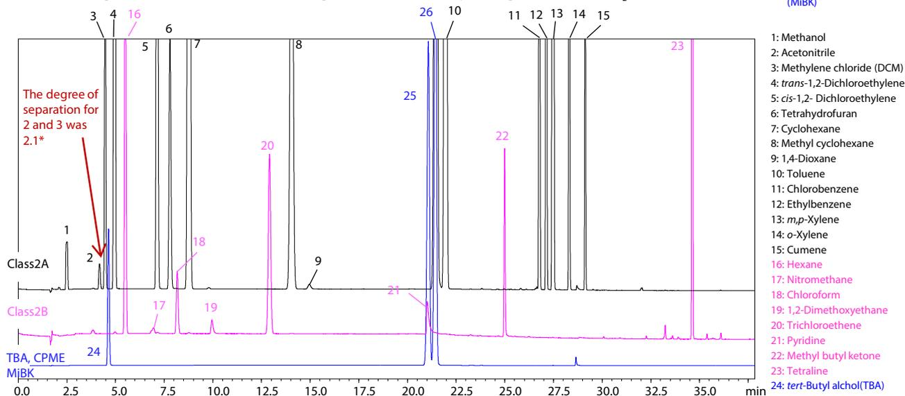
Fig. 9 Class 2 Standard Solution Chromatogram (Water-Soluble Sample) Using Procedure A with H<sub>2</sub> Carrier Gas
