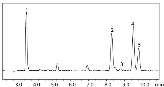
Fig. 6 Class 1 Standard Solution Chromatogram (Water-Soluble Sample) by Procedure A Using N<sub>2</sub> Carrier Gas
