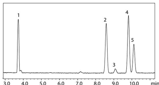
Fig. 7 Class 1 Standard Solution Chromatogram (Water-Soluble Sample) by Procedure A Using H<sub>2</sub> Carrier Gas
