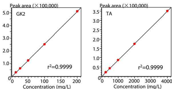
Fig. 3 Calibration curves of GK2 and TA
