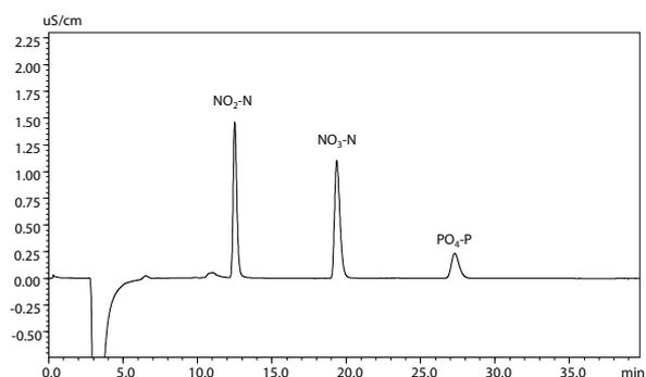
Fig. 2 The chromatogram of mixed standard solution (STD 4: 100 μg/L each)
