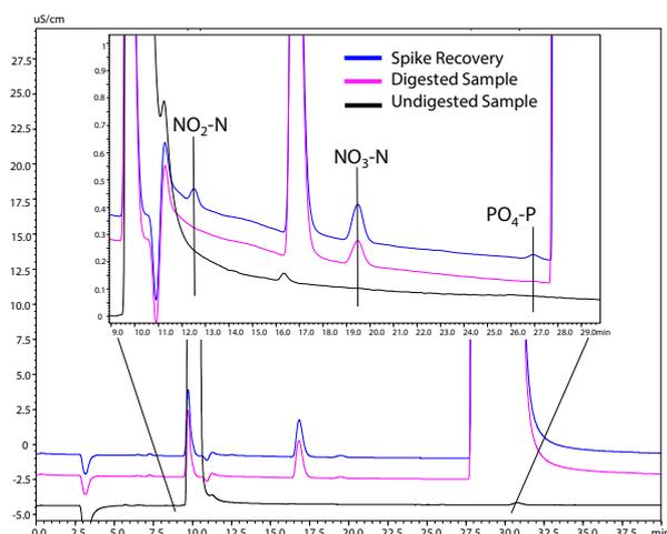
Fig. 5 The chromatogram of undigested sample, digested sample and spiked sample (Diluted 30 times after digestion)
