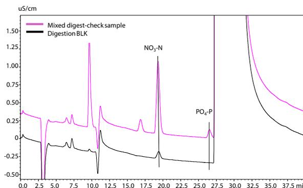
Fig. 4 The chromatogram of digestion blank and mixed digest-check sample (Diluted 30 times after digestion)
