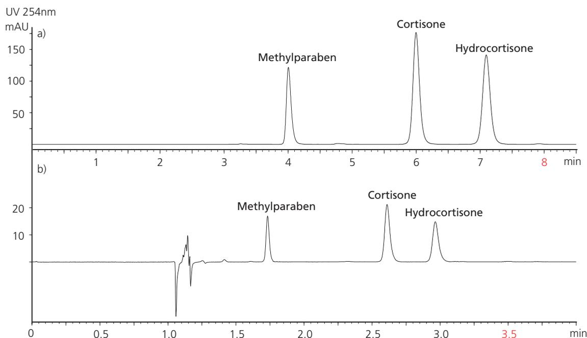
Figure 2: Chromatogram of system suitability solution with a) the USP method and b) the SFC method with conventional column
