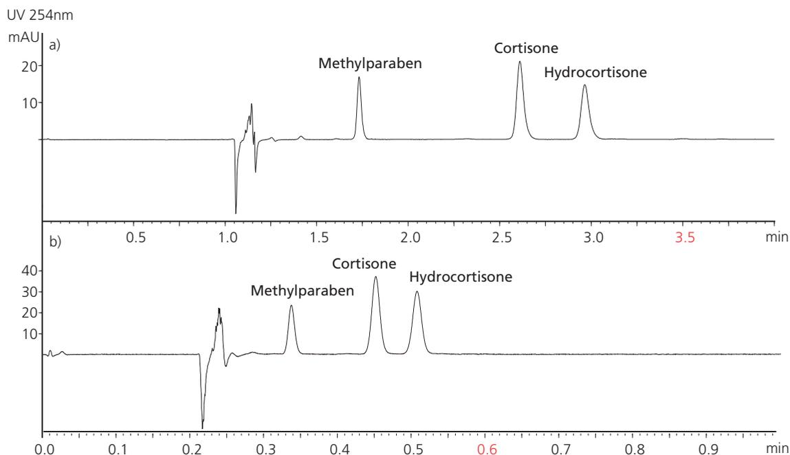
Figure3: Chromatogram of system suitability solution with a) SFC method with conventional column and b) SFC method with UHPLC column
