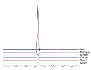
Figure 2: Chromatograms of nicotine standards. The blank was run after the 1000ppm triplicate runs
