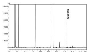
**Figure 3**: Example chromatogram of the e-liquid sample. The other major peaks are likely to be methanol (solvent), propylene glycol and glycerin
